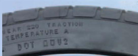
Unfortunately, some manufacturers place the full D.O.T. number on the inner side of the tire—the side facing the *inside* of vehicle. In those cases, only a portion of the D.O.T. number will be on the outer-facing side of the tire, like this:
